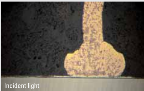
Result: Target prepared integrated circuit. Gold wire bonding on Si .... 25 \mu\text{m} section (LM image)
