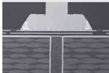
PCB cross section with soldered pin
